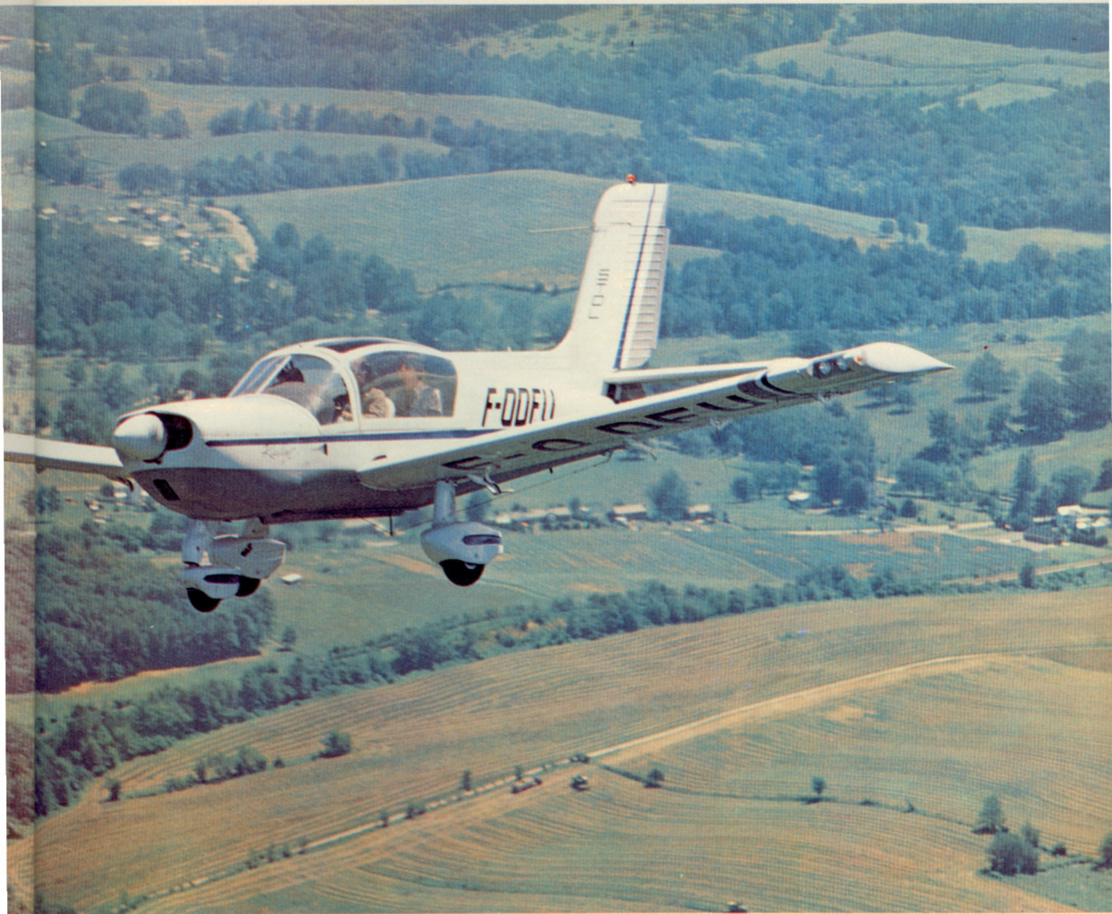
The Rallye 235 GT: its sliding canopy offers a wide-screen view out the side. Photo by Marvin Ickow.
