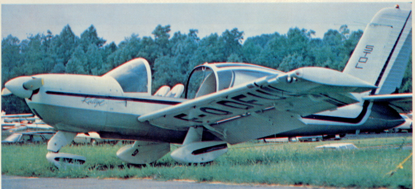
The slats that span the wing's leading edge extend out to 7 inches, and are attached by supports that move on nylon rollers. Narrow chord of wing and large fowler flap can be seen below.
